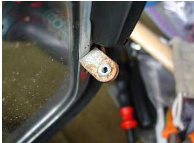
1. Carefully grind off the back of the rivet. You can see that I've protected the glass from accidentally glances from the grinder with a strip of metal sandwiched between two pieces of cardboard. Even so, you need to be very careful with the grinder. A Dremel tool probably will work best in this situation.
