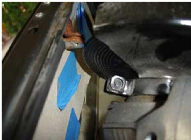
2. Drill the center of the rivet out taking care not to enlarge the opening in the supporting arm by using the appropriate drill bit (I forgot the size I used, sorry - the hole is 4mm iirc). You'll find it easiest to access the rivet if you open the window slightly.
