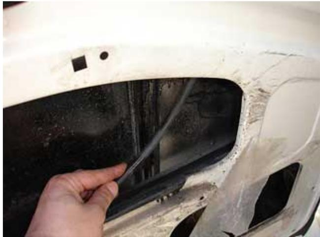
3. With the plastic tube free, tilt the regulator into this position using one hand on the left and the right hand on the plastic tube.
