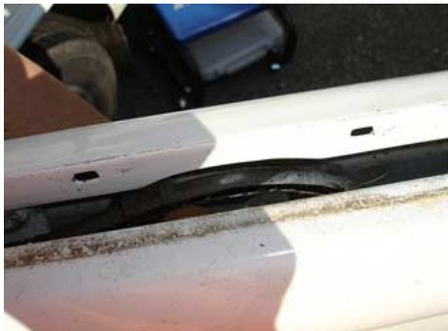
This will allow you to raise the regulator cable plastic tube and free it from the hole that holds it in place.
