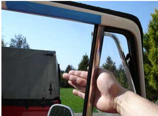
5. Here's the hard part. With the window tilted back slightly, start to lift the vent window assembly from the door letting the top clear the top of the door on the inside.
