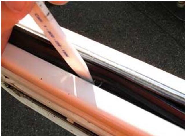
4. At the end of the scraper there is a section of rubber that is wedged between the post of the vent window and the door. If you aren't replacing the inner scraper with a new one, be careful not to tear any rotten rubber there. Use your window tool to put it free. Seal lubricant sometimes helps especially upon re-installation.
