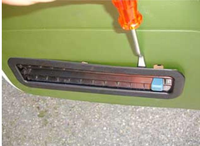
6. Removing the door panel is a matter of levering the 21 trim panel clips that hold the panel to the door. Use your trim panel tool to pop the panel free at each location as you work your way around the edge. Start At the top right corner and work your way clockwise to free the panel. This will keep the panel in place and you can grab hold of it as you release the last few clips along the top.
