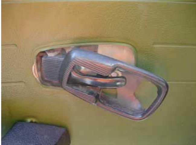
4. The next step is to remove the arm rest. On late model Westys the arm rest is held on by three phillips screws accessed from below. The earlier models had a separate door pull held on with two screws just like the non-Westfalias.
