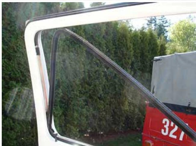
3. The felt clips are held in place by a small tab. The entire clip is made from spring steel but you will find that the tab is not very durable and has a tendency to break. The felt clips can be replaced if they are broken. If you don't have replacement parts on hand I would leave them in place unless you need to remove the outer scraper in which case they must come out.
