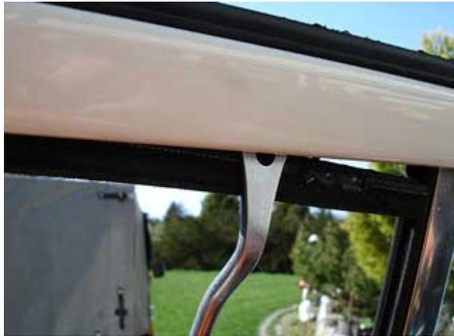
2. As you free the channel from the clips, pull it down from the top and then work to free the section at the side.
