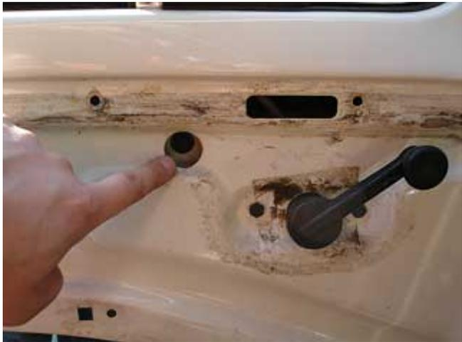
2. Before trying to yank out the window, remove the screw hidden above in the channel where the felt channel is installed. Use a #2 phillips to remove it.
