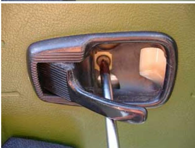
Pulling on the door handle lever, slide the escutcheon to the right to free it. Bag these loose items with the window winder parts.
