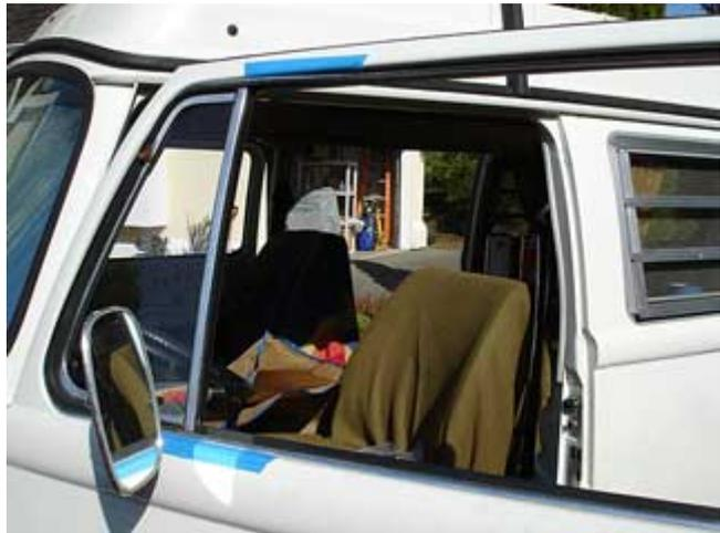
4. With the tape in place and the fasteners removed, use your hand to knock back vent window a couple of inches.
