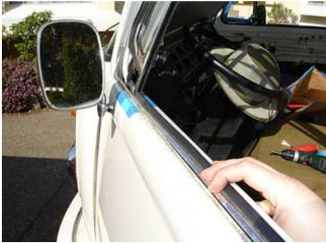
2. Work your way up and down the scraper using the window tool to release it then lift it out of the channel in the door.
