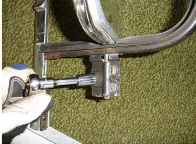
5. With the clamp undone you can pull the quarter-lite from the top by sliding the pivot pin through the opening in the frame. Look at that clamp: there's a good example of the galvanic corrosion that can occur when dissimilar metals touch.
