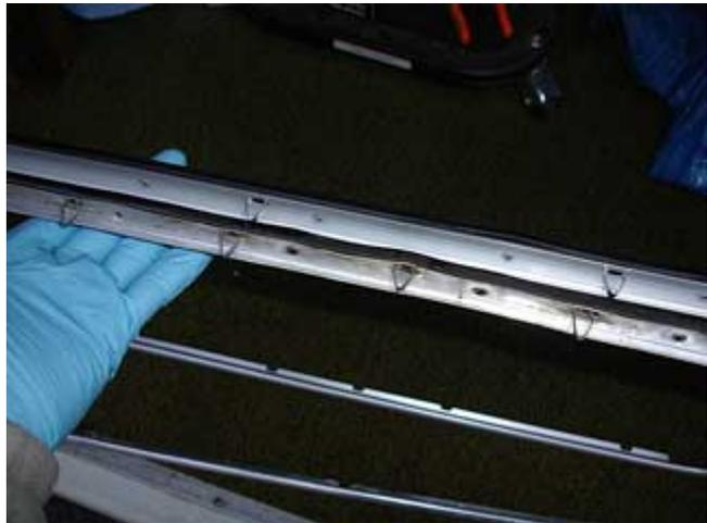
Here's a subtle design difference between the scrapers: this tab at the vent window end of the scraper is flipped around. Both fit.
