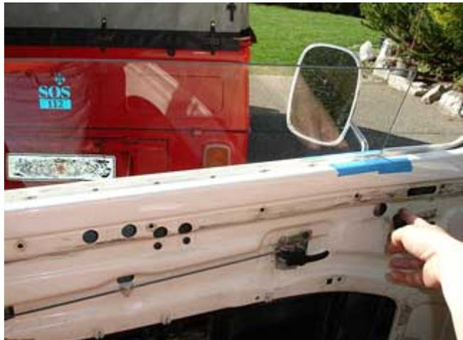
Where is the painter's tape protecting the window I talked about earlier? It should be on the window edges at this point because the barbs on the felt channel clips can scratch the glass as you raise the window.
