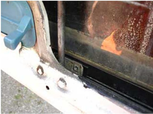
3. To remove the inner scraper use your window seal tool and wedge it between the lip of the scrapers and the door frame. As you do a clip will start to appear and begin to pop out from its notch. Work your way up and down the scraper to release all of the clips.
