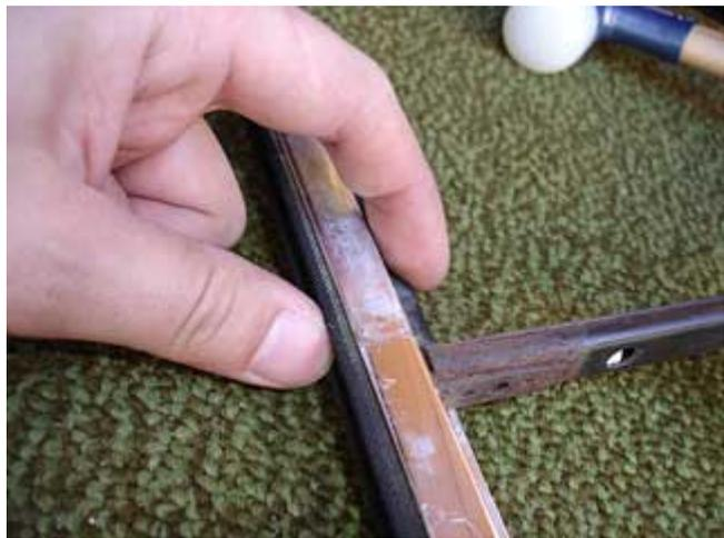
The seal of the inside of the frame and the window channel on the outside should be replaced if they are in poor condition.
