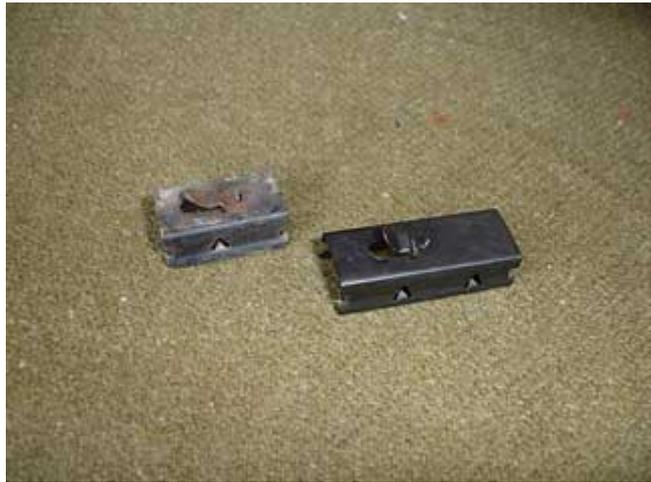
The replacement inner scraper has clips that are stouter than the originals and they are not bent in the same way. This can make it a little harder to re-install and I found that the window seal tool was essential for bending them into position as I pushed with my hand.
