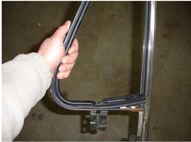
You'll find that the seal has a complicated shape and it will be difficult to fully seal in its groove. You can see the bulge on the seal in this photo and it is supposed to catch in the frame's groove. I used the window seal tool to push the seal into position all the way around. Be sure the seal is properly seated or the vent window may bind against it before you can lock it closed.
