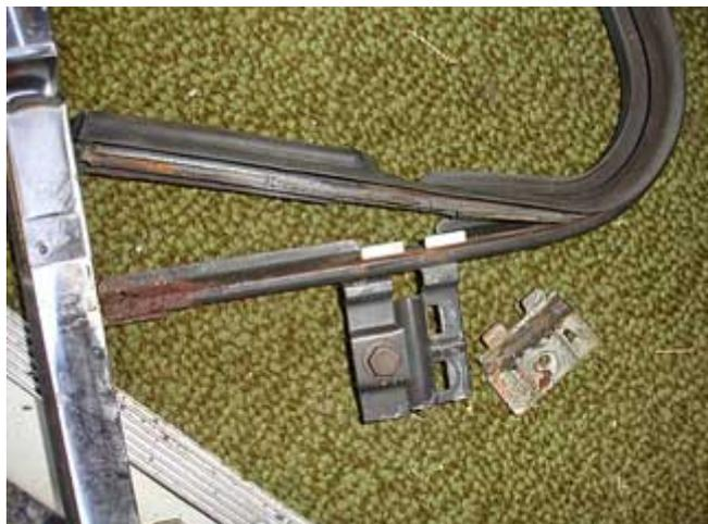
Thread the supporting arm through the seal to remove it completely.
