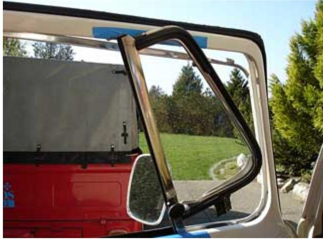
Keeping you from completing your task is this bracket that will not want to twist and get caught on the inside of the door. Watching that you don't scratch anything you have to pull the vent window out of the door using a combinations of wiggling and lifting and tilting. The angle that you have to remove the window is awkward (as seen in the picture above) so be patient and the assembly will eventually lift free.
