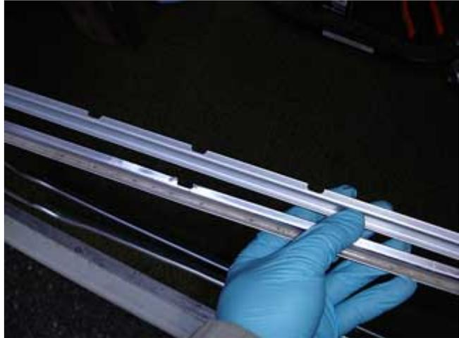
The outer scraper also has fewer clips than the original. I found that the new scraper fits securely with its fewer clips so this is not an issue.
