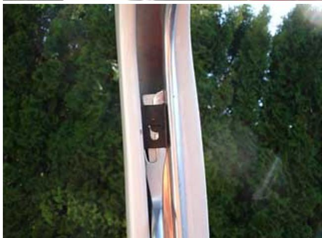
Sometimes the clips come out by prying on them a little and other times they have to be tapped with a punch and hammer before coming loose. Be careful with the tab and take note of the orientation of the felt clips for re-installation.
