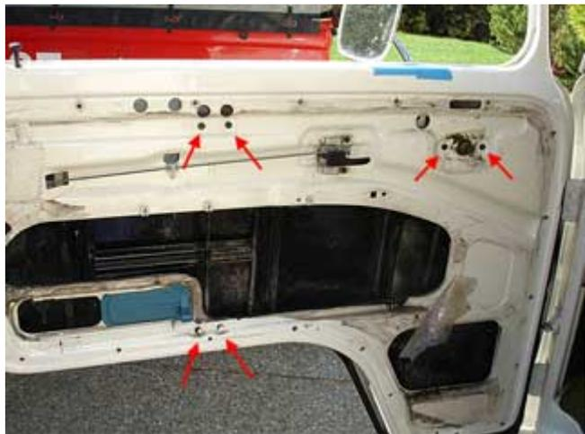
2. Lift the regulator slightly on the vent window side of the door.
