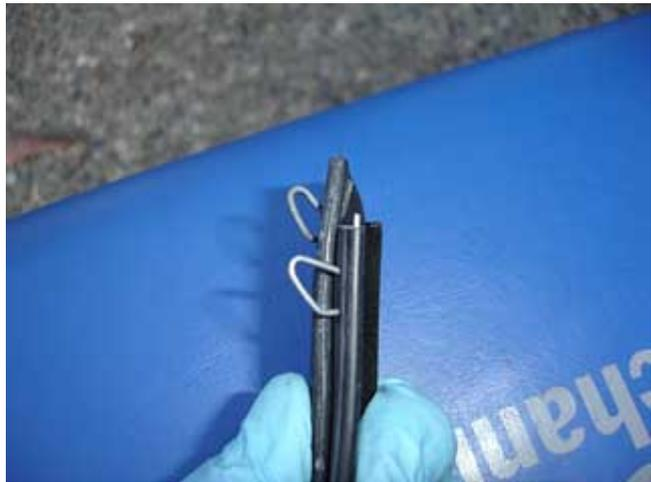
Another problem with the inner scraper is that the profile has changed. Since my inner scraper wasn't in bad shape and on the inside of the window anyway I elected not to replace this part and kept the original.
