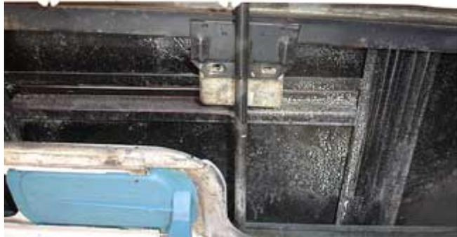
2. Wind the window up. Without the window scrapers and with the window lowered you will have to guide it through the opening as you initially wind it.
