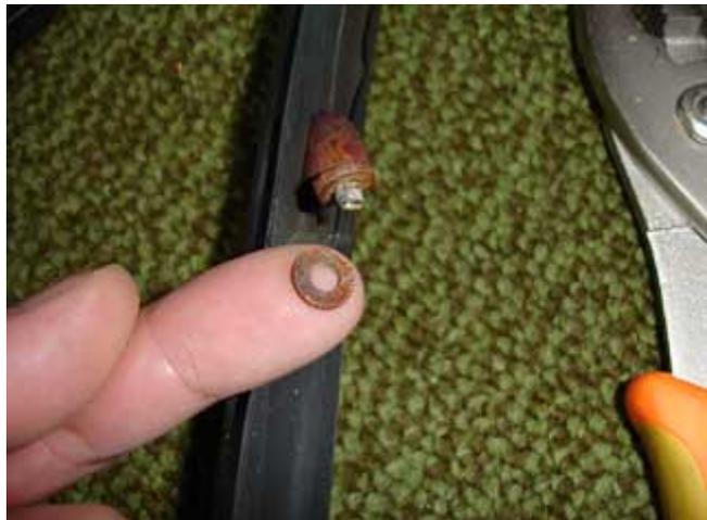
4. Undo the adjusting clamp bolt using a 13mm socket wrench. After removing the bolt and washer (bag 'em) kick yourself (ouch!) for not remembering how many turns of the screw were required to set the tension on the clamp.
