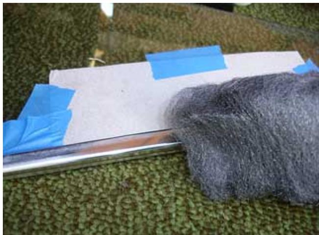
So long rust! I used a stainless steel brush to get rid of the rust and a little help from the flap wheel on my grinder. This is bare metal now so it has to be covered with clear spray paint or it will rust all over again.
