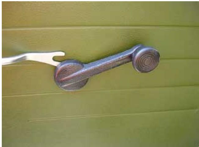
With the screw removed the window winder will pull straight off and the black window buffer behind it will drop free as well. Save all of these items in a Ziploc bag for reassembly later.
