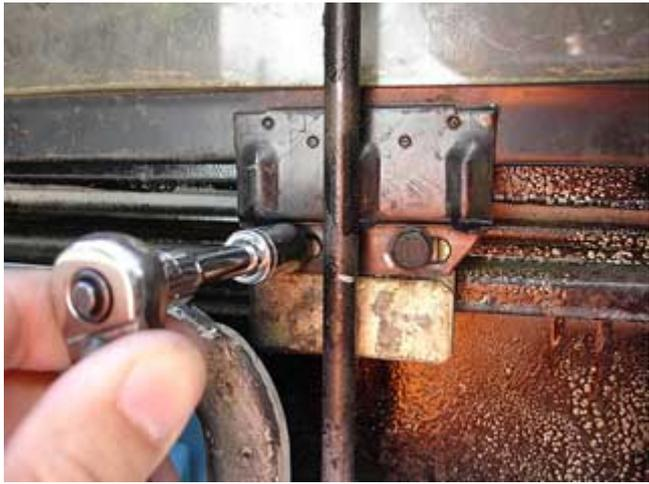
2. With the bolts removed you can wind the window back down to the bottom and then lift the window up by the lift channel (support bar) and then carefully lower it behind the bracket letting it rest of the bottom of the door.
